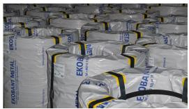
Ecofix, high-quality steel straps are produced by Ekobant Metal. It's a steel strap manufactured with the highest technology full automatic production line which starts with cold rolling of low-medium carbon steel, heat treatment of high carbon steels with a stress relief process and ends with packing. Upon customer request blue tempered, black painted, bright and waxed surfaces can be created.
